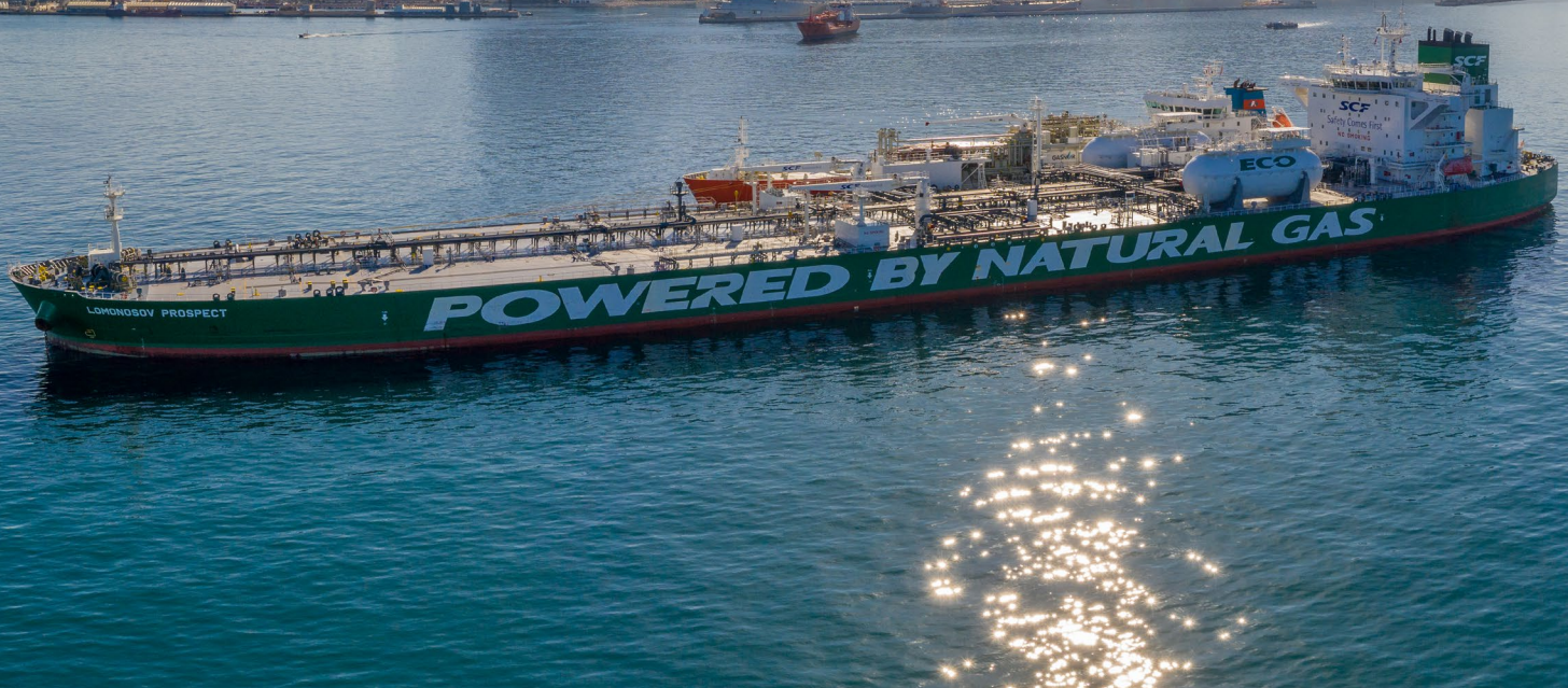
The tanker Lomonosov Prospect using LNG as the primary fuel during LNG bunkering in Gibraltar.
